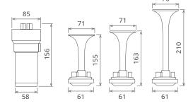
No need for an air tank on board. Kit includes heavy-duty compressor, relay, hose and mounting hardware. Harmonic sound with three trumpets made of durable plastic with colour of red or chromium plated. Available with 12V or 24V
