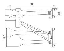
Our new 85KH compressor air horn has the top quality and powerful sound. Moreover, it is cheaper than equivalent compressor air horns of other European brands (European made). Double sound, two metal trumpets of chrome coating. Trumpets are 26cm and 34cm. No need an air tank on the vehicle because 85KH has its own air compressor. Available as 12V or 24V.
