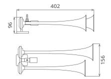
Single blasting sound, two trumpets (sound typology changes according to number of trumpets). Single solenoid type, only for vehicles equipped with an air tank on board. Available as 12V or 24V. Trumpets are in aluminium, colour may be red or chrome.
