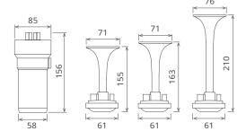
No need for an air tank on board. Kit includes heavy-duty compressor, relay, hose and mounting hardware. Harmonic sound with three trumpets made of durable plastic with colour of red or chromium plated. Available with 12V or 24V
