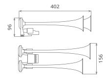
Outstanding alternate sound (2 sounds), two trumpets (sound typology changes according to number of trumpets). Double solenoid, with an electronic circuit also. Only for vehicles equipped with an air tank on board. Available as 12V or 24V. Trumpets are in aluminium, colour may be red or chrome.
